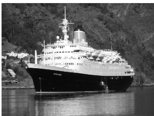
' Saga Rose ' Saga Holidays Ltd. 24,528 GRT. L.o.a. 189m. Bm. 24m. Kts. 20. Passengers 587
