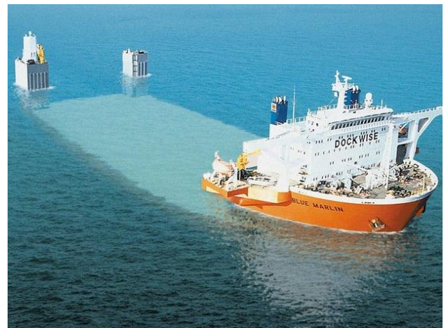
Blue Marlin submerging to accept a heavy lift. Courtesy of Imgur.Com
