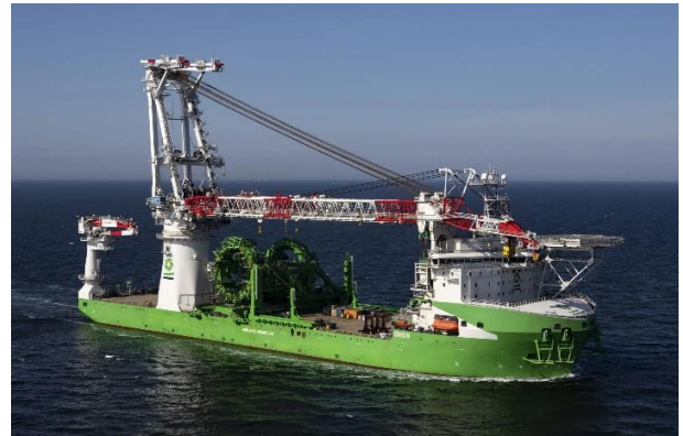
DEMA Offshore Heavy Lift DP3 Installation Vessel Crane Capacity - main 5,000 ton - aux 1,500 ton
