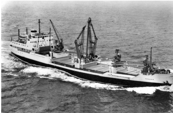
TJ Harrison's 5,788grt Trader was built in 1966 by Lindholmens Varv at Gothenburg. (John B. Hill collection) her Stulken was capable of lifting 70 tons.
