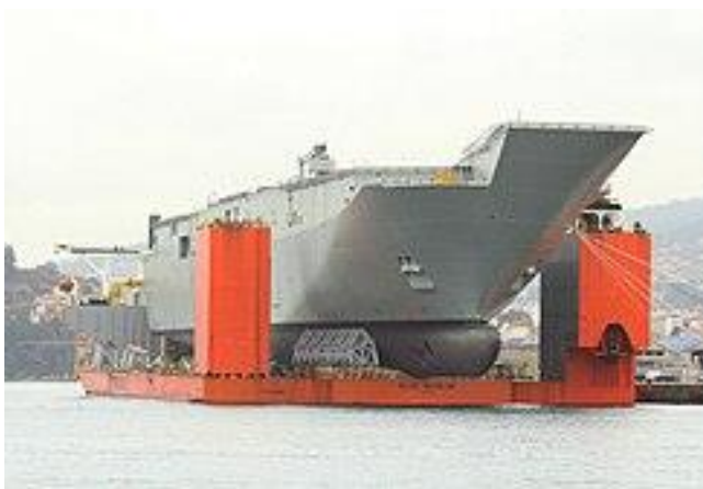
The incomplete Australian landing helicopter ship HMAS Adelaide on Blue Marlin
