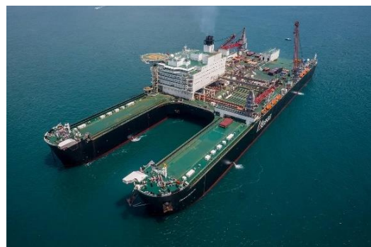
And... The world's largest heavy lifter Allseas Group's Pioneering Spirit capable of lifting topsides up to 48000mt and jackets up to 25000mt.
