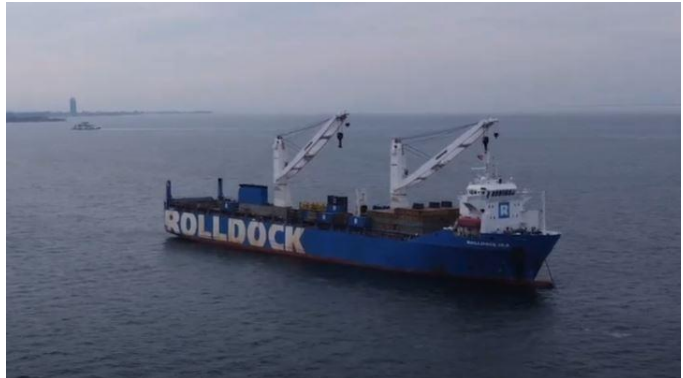
Rolldock – S Class (Sun, Sea & Sky) with Ro-Ro Stern Ramp with a capacity up to 4,000 mt unit weight depending on cargo configuration. 2x350 mt Liebherr Cranes (combi 700 mt) with an outreach of 350 mt at 18 m & 200 mt at 33 m. She also has an auxiliary hoist of 45 mt at 36.2 m.
