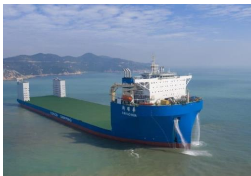
Xin Yao Hua capable of loads of 25tons/m 2 & overall 125ton/m on webframes – from Cosco site.
