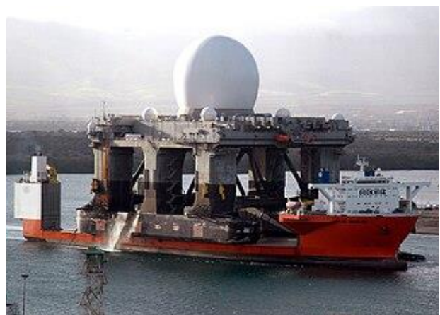
Blue Marlin carrying the Sea-Based X-Band Radar
