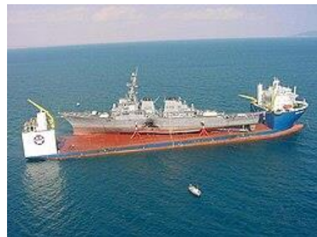
Dockwise Limited's Blue Marlin - semisubmersible heavy lifter with a carrying capacity of up to 75000mt. Seen here with the USS Cole (max displ. 8300 tons)
