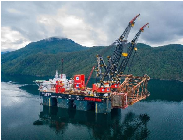
Sleipnir with the 8100 ton Jotun B jacket suspended in its cranes for deliver to recycling
