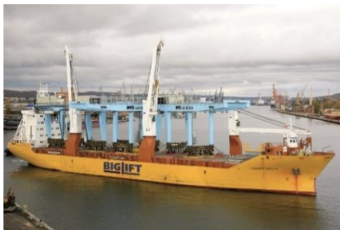
BigLift's Happy Delta - flexible, heavy lifters with two Neuenfelder Maschinenfabrik (NMF) cranes with a SWL 400mt and one NMF crane SWL 120mt.
