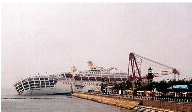
Immediately after the storm passed through Dalian after being holed on her port bow and lower decks flooded
