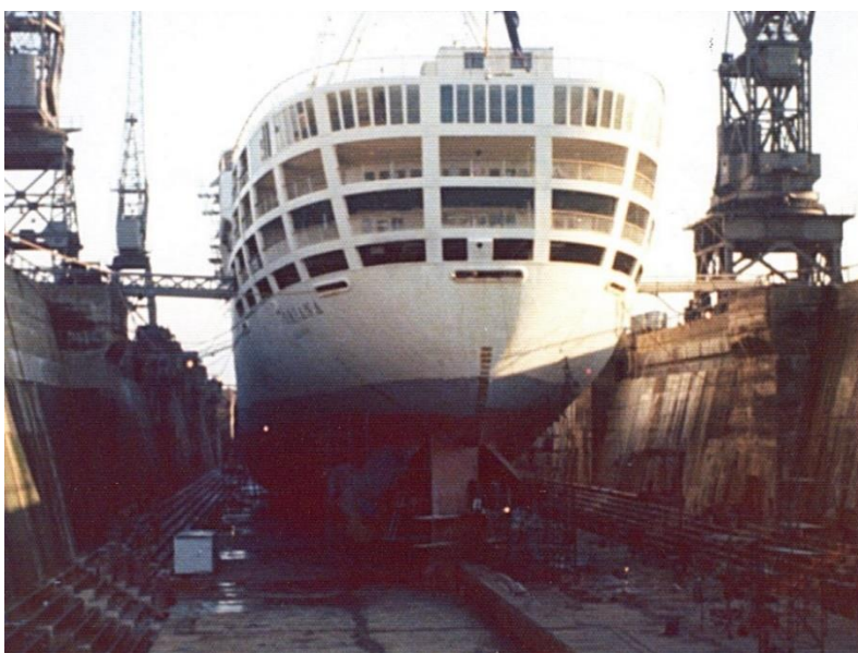
Oriana props removed for the fitment of the new 'Eco-Props' and David's chunk of the old!
